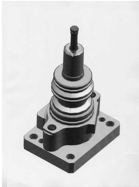
The two machine components above can only be assembled in one way, the correct way: the poka-yoke design eliminates the possibility of assembly mistakes.
