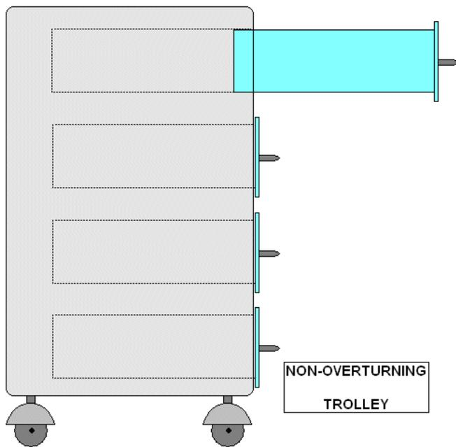
Filing Cabinets, Tool Cabinets and the like could overturn if all drawers are open at once. But if only one drawer at a time can be open, the possibility of overturning is eliminated.
