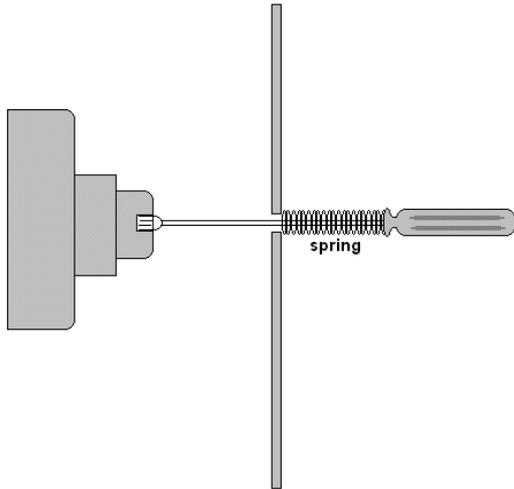
In the example, a machine needed to be set-up rather often: to the purpose, a technician would use a socket screwdriver, inserted through a transparent cover.
